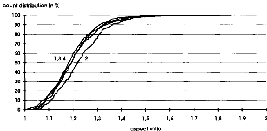
Fig. 5. Count distributions of aspect ratio for fluid-bed-dried (1), oven-dried (2), freeze-dried (3) and wet (4) pellets of formulation ace2.3.
